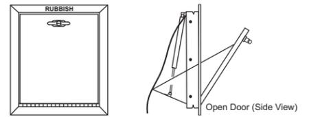
Doors are constructed entirely of type 304 stainless steel with stainless hinges. Doors are bottom hinged, self closing and self latching with a locking Tee handle. UL class B labeled: 1 1/2 hour fire rated with 30-minute temperature rise of 250° F. Door trim embossed "RUBBISH".
