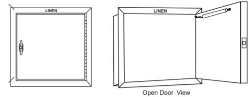
Doors are constructed entirely of type 304 stainless steel with stainless hinges. Doors are side hinged, self closing, and self latching with a locking Tee handle. UL class B labeled: 1 1/2 hour fire rated with 30-minute temperature rise of 250° F. Door trim embossed "LINEN".
