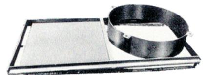
Horizontal rolling type discharge door assembly, required when chute discharges into an open container. Gravity rolling door held open with a UL approved 165° fusible link.
